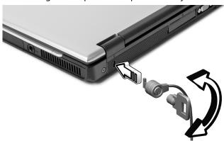
Wrap a computer security lock cable around an immovable object such as a table or handle of a locked drawer. Insert the lock into the notch and turn the key to secure the lock. Some keyless models are also available.
